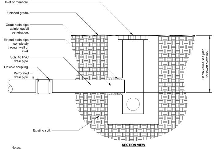
1- Invert of the drain line (bottom of the pipe) shall be above the top of the out fall pipe unless otherwise indicated on the drawings.
